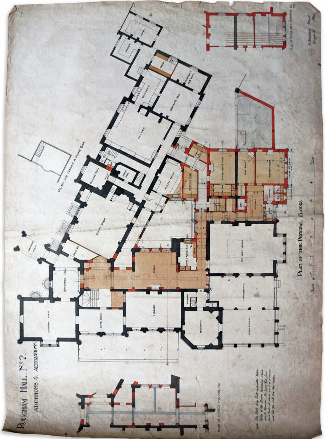
FIG. 161 – Ground floor plan of Rougham Hall showing the alterations proposed by the architect John Macvicar Anderson in 1904. (Courtesy of the Rougham Estate Trust).
